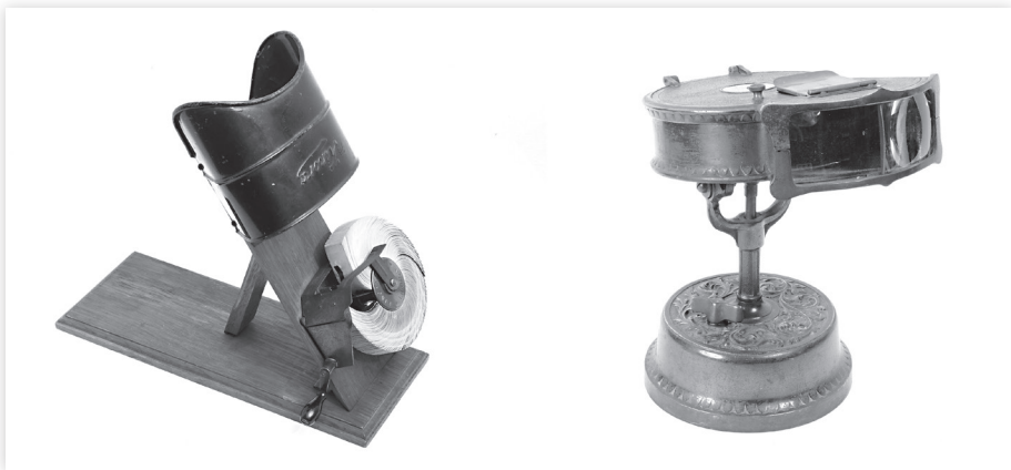
Figure 4. Kinora viewer: basic wooden model with single window (left) and cabinet viewer with multiple windows (right). Photos © Antiq-Photo Gallery, Paris.
